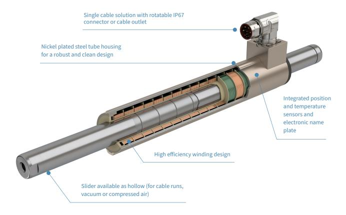
LinMot P01 linear motors are permanently actuated ironless synchronous servo motors with integrated position measurement and over-load protection. Powerful rare-earth magnets in the slider and windings in the stator are used to directly generate the linear motion.
