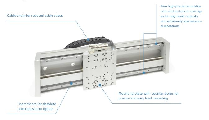
Our moving stator linear guides offer a high guidance accuracy, a precise load positioning and a reliable operation even with heavy loads and over a long distance. They consist of a special aluminium profile on which up to 2 high precision rails with up to 4 linear ball bearing carriages can be mounted.
