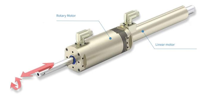
The PR01 product family combines a linear and a rotary motor in just one housing. The two electromagnetic servo motors are built in series and thus enable the installation of this machine element in the smallest possible footprint. Numerous options such as the MagSpring load compensation, pneumatic brake, emergency rail kit and wiper can be added to the module.
