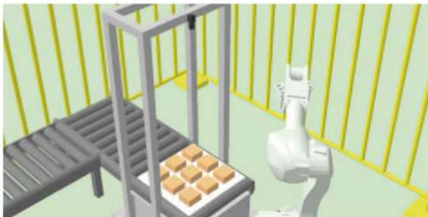
Picking of workpieces on a pallet after positional measurement
