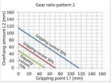
Even if the gripping point distance is within the limit range, keep it as small and lightweight as possible. If the fingers are long and large, or if the mass is large, inertial force and bending moment during opening and closing may worsen the performance and adversely affect the guide section.
